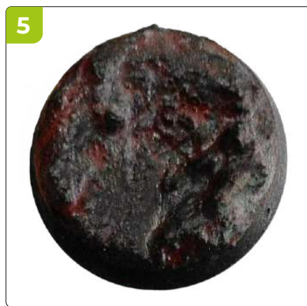
5. RUST - Light Rust
